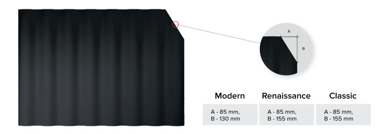
The size of the cut corners rests on the most common shape roof, the angle of inclination of which is > 30° (Modern - overlapping of the sheet 125 mm, Renaissance and Classic - 150 mm). If the angle is smaller, the value leg B along the slope increases according to DBN (State Construction Standard).
