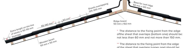
\*\* The distance to the fixing point from the edge of the sheet that overlaps (upper one) should be: not less than 65 mm and not more than 140 mm. In some cases, it can be more than 140 mm if the sheets overlap is more than 200 mm.
