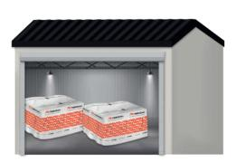
Fiber cement sheets and its accessories are to be stored in closed dry warehouses on wooden pallets or rails and covered with branded packaging until fully used.
