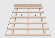
If needed, a waterproofing film is used. It spreads along the rafters and fixes with a truss.The distance between the centers of the lathing depends on the roof inclination angle.The rafter cross-sectional dimension depends on its length (L) and the distance between the rafters (A).
